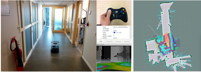
Fig. 6: The human-in-the-loop experiment setup, where the robot is controlled by both its autonomous controller and the human inputs.
