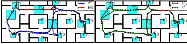
Fig. 2: The robot's trajectory in simulation case One, where the robot's initial plan is in blue, the human-guided part is in red, and the updated plan is in green.
