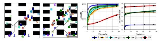
Figure 2: Left two: Snapshots of simulated systems of 5 (left) and 10 (right) robots. Robots are denoted by green circles with battery level indicated by blue bars. Charging stations are marked by blue arrows and shelves are in black. The loading and unloading location of a transportation task are marked in filled and checked squares. Right two: Evolution of episode length (left) and degree of intervention (right) of the safety network for system with 5, 10, 15 robots.
