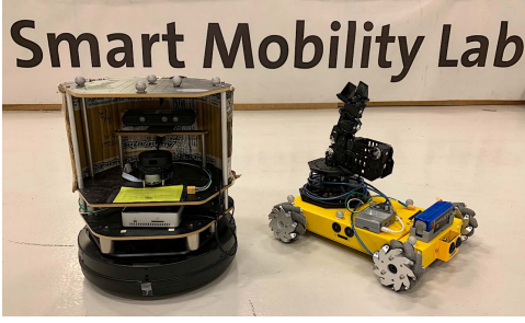
Fig. 1. TurtleBots (left) and Nexus 4WD Mecanum Robotic Cars (right) are used in the experiments in Section IV.
