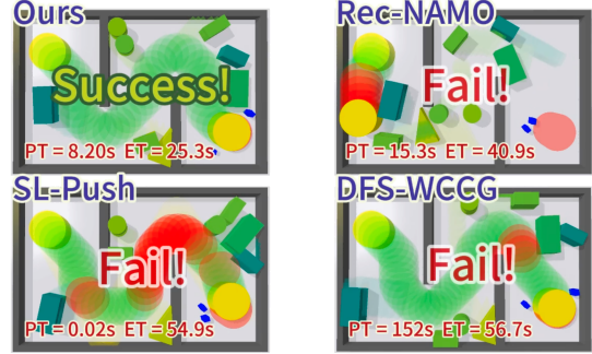
Fig. 8. Failure cases by baselines Rec-NAMO, SL-Push and DFS-WCCG.
