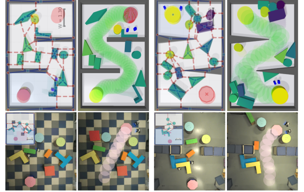
Fig. 1. Collaborative path clearing in simulation (Top) and hardware (Bottom). Two robots push movable obstacles to create a W-clear path for a large vehicle from start to goal.
