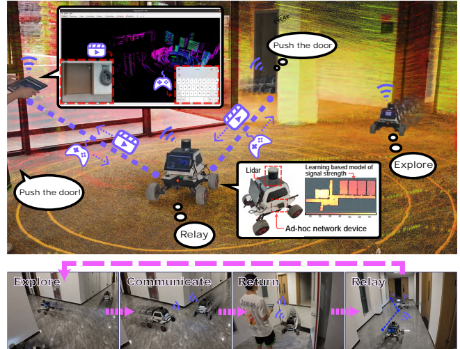
Fig. 1: Top: the FlyKites system deployed for hardware experiments. One robot explores the workspace, while two robots in relay mode to transmit: (I) live video stream from the end robot to the operator, and (II) tele-operation from the operator to the end robot to open a door. Their communication is fully distributed via ad-hoc networks, of which the quality is predicted via a learned model. Bottom: Three UGVs transit between exploration, intermittent communication, return to the operator, and communication relay.
